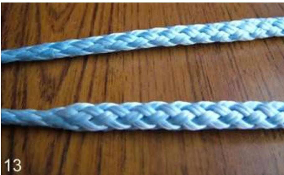
The lower spliced rope shows the effect of not tapering the working end prior to burying it inside the rope. There is a sharp change in diameter, which can weaken the splice. This is absent from the top rope, which has been tapered properly. These ropes and splices are exactly the same diameter but the
