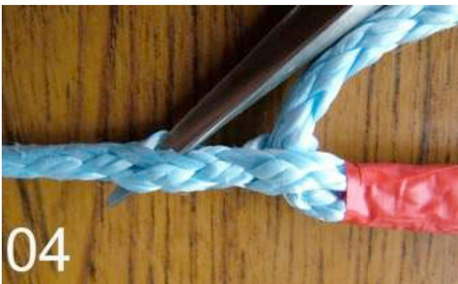
The next step is a fiddly one. When you open up the rope by pushing along its axis you can see little holes where the strands open up. Skip two holes, from the exit point of the first tuck, and push the fid into the third hole at an angle of about 45 degrees, as in the picture. This means that it should come out at the fourth hole on the under side. That's the fiddly bit
